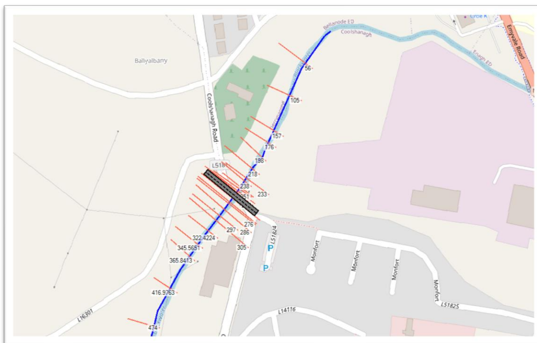
Figure 4 1D Flood Model Schematization
