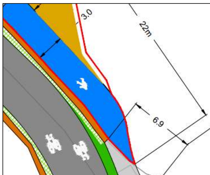
Figure 2-4 – Proposed end of wall/ Parapet
