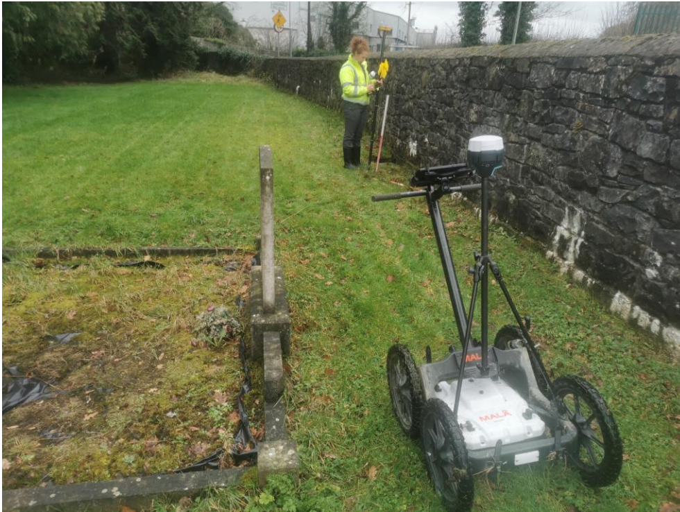
Figure 5: GPS surveying with the GPR cart in the foreground.
