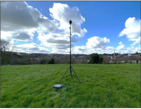
Figure 2 Noise Measurement Location 1 (Unattended)
