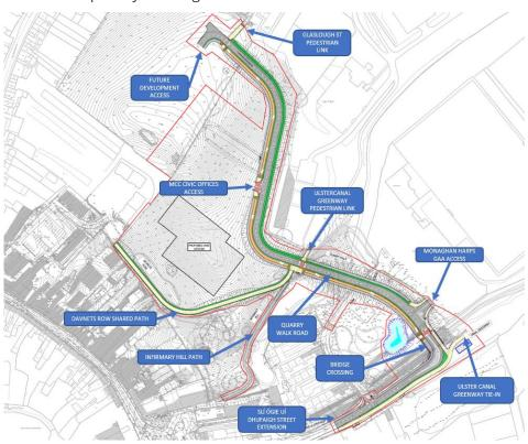
Figure 14 Overview of Road Access and Active Travel links (Source: DBFL Infrastructure Design Report).
